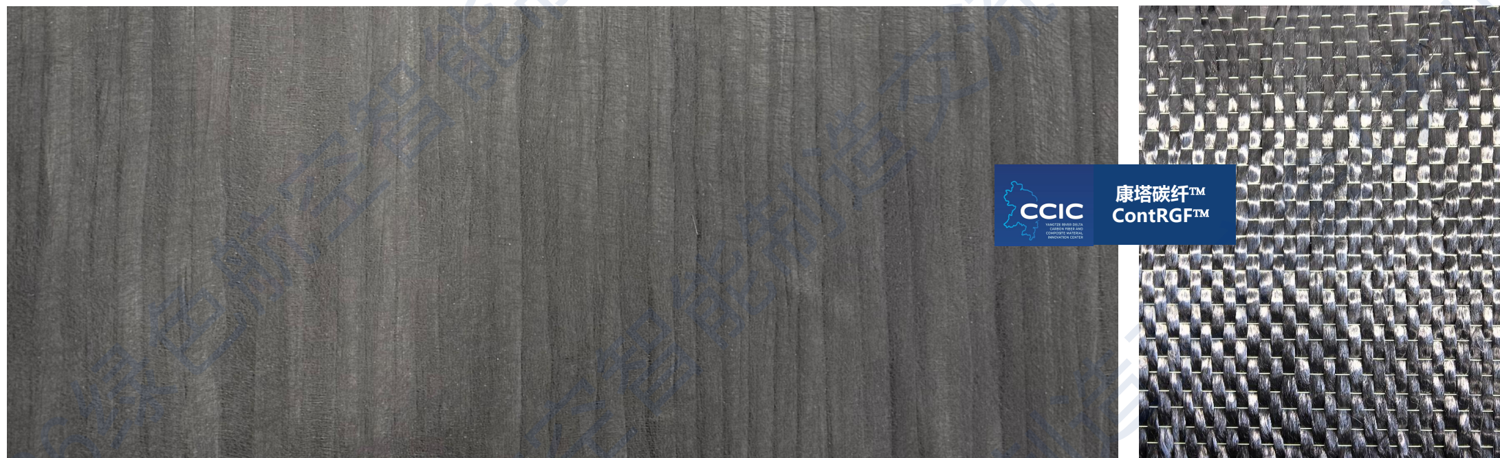
康塔碳纤™的典型面密度 (24k) / Typical areal density of ContRGF™: 200g/m 2 ~ 1000g/m 2
