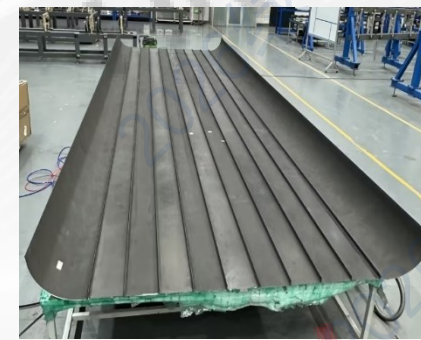
中机身上壁板尺寸: 8.27m*2.6m*0.31m 共固化工艺
