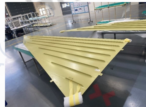
中机身上壁板尺寸: 8.27m*2.6m*0.31m 共固化工艺
